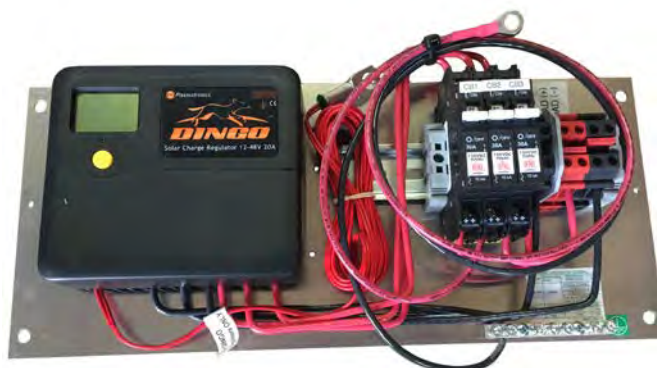
PRE Control Panel with a 20 amp DINGO
