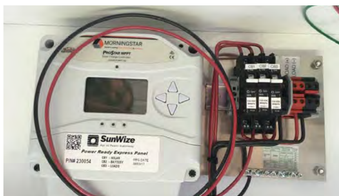
PRE Control Panel with a 25 amp MPPT ProStar with meter
