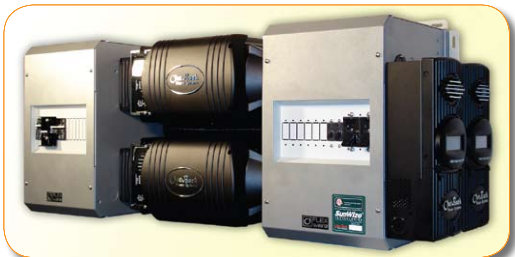
The FW500 inverter power centers are assembled and tested at SunWize to UL-508A listing for USA and Canada CAN/CSA 22.2#14-M95 "Industrial Control Panel". Shown with two OutBack GVFX inverters/chargers, two FM60 controllers.
